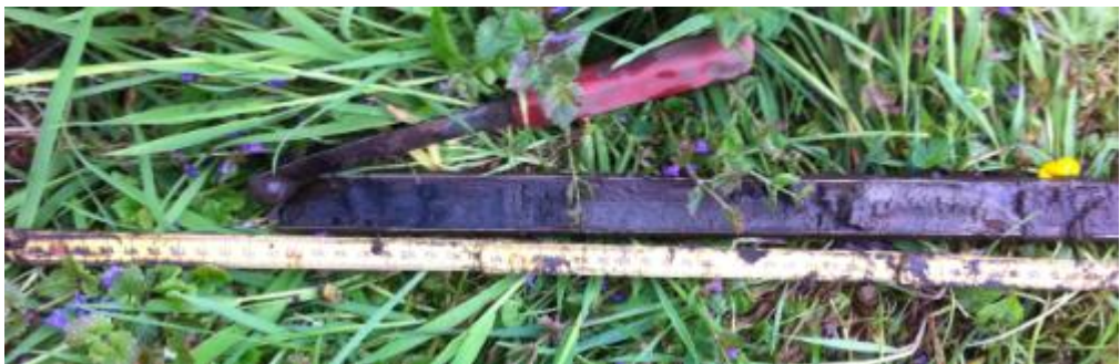
Boring 6: detail gutskern onderkant boring.
